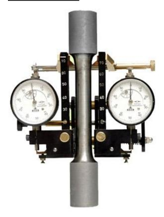
**DESCRIPTION:** An extensometer is a device that is used to measure changes in the length of an object. It is useful for stress-strain measurements and tensile tests
