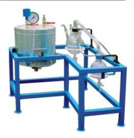
**DESCRIPTION:** The equipment consists of Borosilicate glass round bottom flask as distillation still. The distillation is carried out by using steam. The vapors coming from the column is going in to the condenser. The distillate is collected in round bottom flask.
