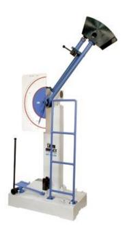
**DESCRIPTION**: The Charpy impact test, also known as the Charpy V-notch test, is a standardized high strain-rate test which determines the amount of energy absorbed by a material during fracture. This absorbed energy is a measure of a given material's notch toughness and acts as a tool to study temperature-dependent ductile-brittle transition. It is widely applied in industry
