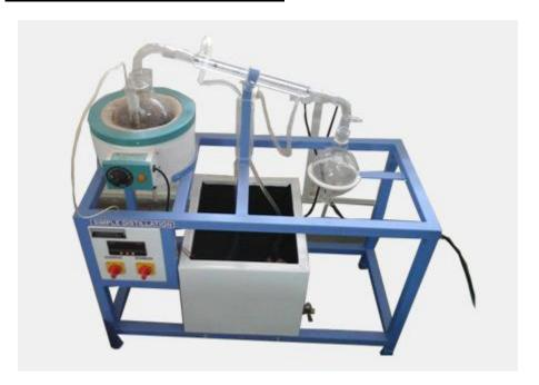
**DESCRIPTION:** The equipment consists of Borosilicate glass round bottom flask as distillation still. The distillation is carried out by heating the still. The vapors coming from the column is going in to the condenser. The distillate is collected in round bottom flask
