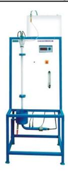
**DESCRIPTION:** A Thin film of liquid running down the inside of vertical pipe, with gas flowing either concurrently or counter currently, constitutes a wetted wall tower. In this the liquid is dispersed into thin film .Measurement of the rate of evaporation of the liquid in to the gas stream over known surface permits calculation of the mass transfer coefficients for the gas phase
