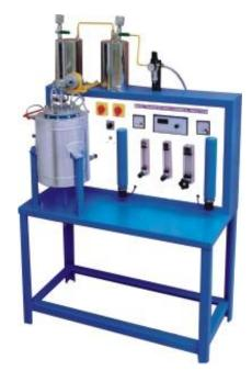
**DESCRIPTION:** In this reactor contents are well stirred with the catalyst and uniform throughout. Thus exit stream from this reactor has the same composition as the fluid within the reactor. We can refer also mixed type reactor
