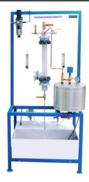
**DESCRIPTION:** The Adsorption column consist of glass column filled with adsorbent. The feed is introduced from the top of the column. The solute from the feed solution is adsorbed on the adsorbent surface. After the operation the solution drain out and analysed. Steam
