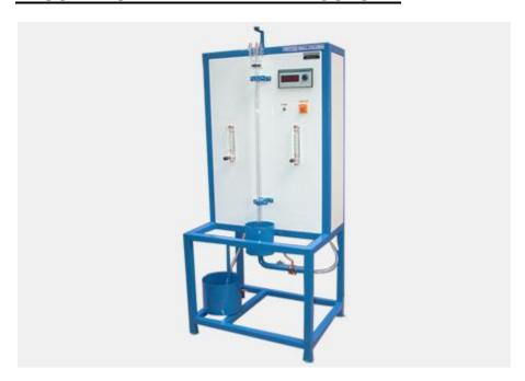
**DESCRIPTION:** The Absorption column consist of Glass column. The device is equipped with a gas inlet and distributing space at the bottom, a liquid inlet and distributor at the top, gas and liquid outlet at top and bottom respectively. The gas and air are metered separately, mixed and then passed through the bed vertically upwards and absorbed in liquid. All the flow rates can be independently varied to simulate different conditions.
