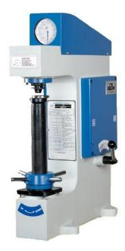
**DESCRIPTION**: The Rockwell scale is a hardness scale based on indentation hardness of a material. The Rockwell test determines the hardness by measuring the depth of penetration of an indenter under a large load compared to the penetration made by a preload. <sup>[1]</sup> There are different scales, denoted by a single letter, that use different loads or indenters. The result is a dimensionless number noted as HRA, HRB, HRC, etc., where the last letter is the respective Rockwell scale
