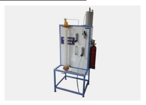
**DESCRIPTION:** The Absorption column is consist of glass column packed with Rasching rings. The device is equipped with a gas inlet and distributing space at the bottom, a liquid inlet and distributor at the top, gas and liquid outlet at top and bottom respectively. The gas and air are metered separately, and then passed through the bed vertically upwards and absorbed in liquid. All the flow rates can be independently varied to simulate different conditions.
