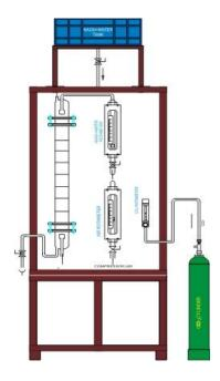
**DESCRIPTION:** The Absorption column consist of Stainless steel column. The device is equipped with a gas inlet and distributing space at the bottom, a liquid inlet and distributor at the top, gas and liquid outlet at top and bottom respectively. The gas and air are metered separately, mixed and then passed through the bed vertically upwards and absorbed in liquid. All the flow rates can be independently varied to simulate different conditions.
