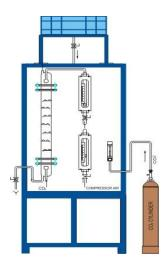
**DESCRIPTION:** The Absorption column consist of Stainless steel column. The device is equipped with a gas inlet and distributing space at the bottom, a liquid inlet and distributor at the top, gas and liquid outlet at top and bottom respectively. The gas and air are metered separately, mixed and then passed through the bed vertically upwards and absorbed in liquid. All the flow rates can be independently varied to simulate different conditions.
