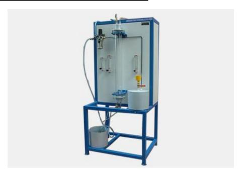
**DESCRIPTION:** The Absorption column should consist of Glass column. The device must equipped with a gas inlet and distributing space at the bottom, a liquid inlet and distributor at the top, gas and liquid outlet at top and bottom respectively. The gas and air are metered separately, mixed and then passed through the bed vertically upwards and absorbed in liquid. All the flow rates can be independently varied to simulate different conditions.
