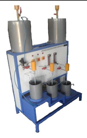
**DESCRIPTION:** C.S.T.R is a reactor in which the content are well stirred and uniform throughout. Thus exit stream from this reactor has the same composition as the fluid within the reactor. We can refer also mixed type reactorThe reactants are initially charged in to a container, mixed well and then left to react for certain period of time. At any instant the composition throughout the rector is uniform.
