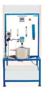
**DESCRIPTION:** C.S.T.R is a reactor in which the content are well stirred and uniform throughout. Thus exit stream from this reactor has the same composition as the fluid within the reactor. We can refer also mixed type reactorThe reactants are initially charged in to a container, mixed well and then left to react for certain period of time. At any instant the composition throughout the rector is uniform.
