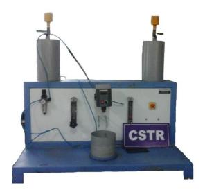
**DESCRIPTION** C.S.T.R is a reactor in which the content are well stirred and uniform throughout . Thus exit stream from this reactor has the same composition as the fluid within the reactor. We can refer also mixed type reactor
