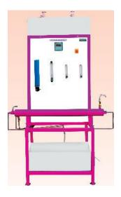
**DESCRIPTION:** Plug flow reactor is characterized by the fact that the flow of fluid through the reactor is orderly no element of fluid overtaking or mixing with any other element ahead or behind
