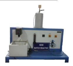
**DESCRIPTION:** Semi Batch reactor is simple, needs little supporting equipment and therefore ideal for small scale experimental studies on reaction kinetics. Industrially it is used when relatively small amounts of material are to be treated.
