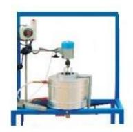
**DESCRIPTION:** Adiabatic batch reactor is simple, needs little supporting equipment and therefore ideal for small scale experimental studies on reaction kinetics. Industrially it is used when relatively small amounts of material are to be treated.
