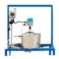
**DESCRIPTION:** Batch reactor is simple, needs little supporting equipment and therefore ideal for small scale experimental studies on reaction kinetics. Industrially it is used when relatively small amounts of material are to be treated.
